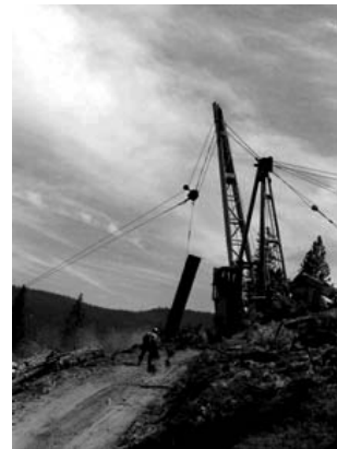
Figure 4. On the left, a ground based log skidder. On the right a cable yarding system, which is used on steep slopes to transport felled logs from the stump to a landing area
