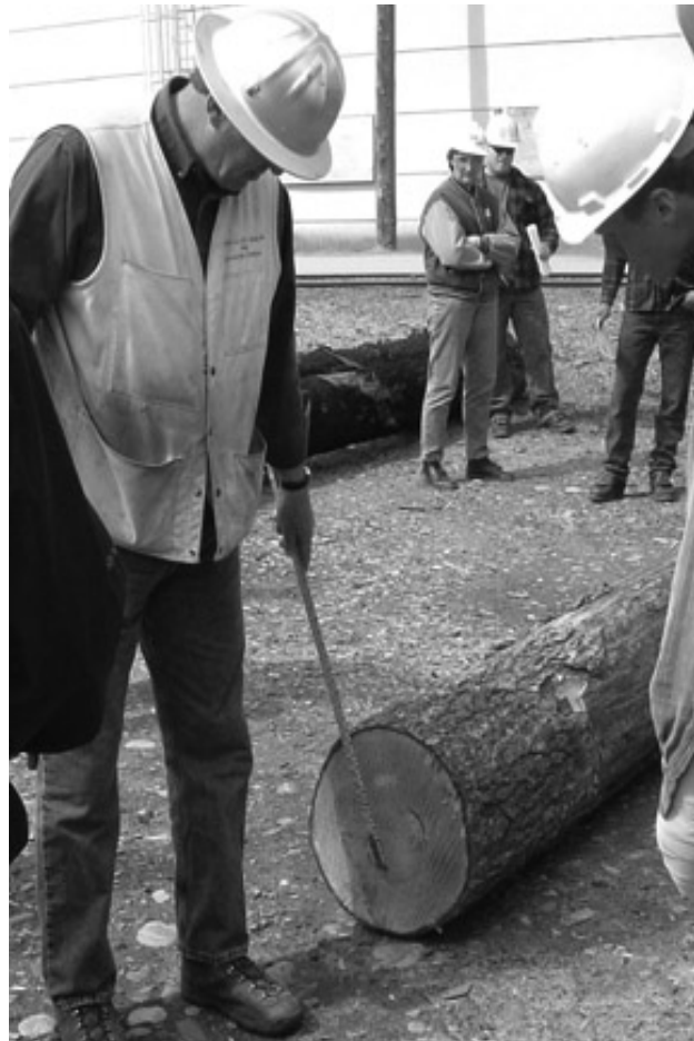
Figure 2. Log scaler measuring log volume and quality
